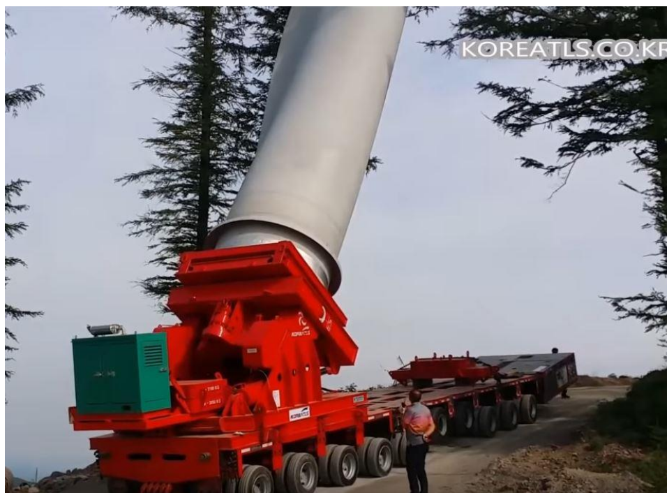
Figure 4.3.13. Special equipment for transporting WPP wings
